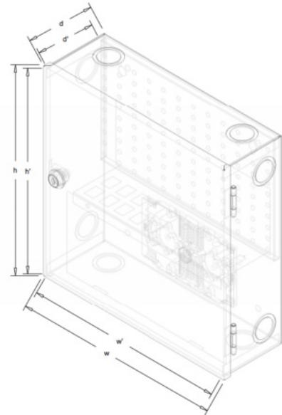
On request we can be made in other dimensions or any number and arrangement blind holes ( $\varnothing 29 / 38$ ) or holes in the panel
